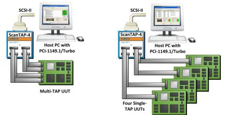
PCI-1149.1/Turbo with ScanTAP-4 Configurations.
